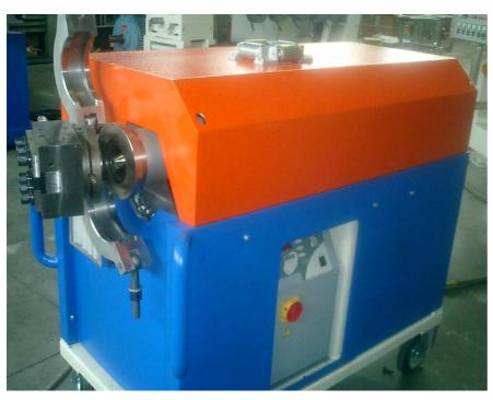
Extruder mounted on wheels for easy positioning
